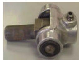
Polished 911 rear shift coupler with new rubbers
