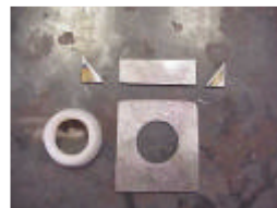
Layout the pieces for the new bushing support
